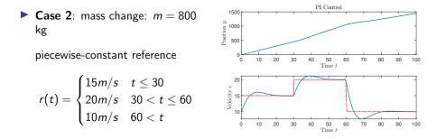
**Robustness**: The same PI controller can make the closed-loop system follow a reference signal even when some system parameters are not known exactly.
