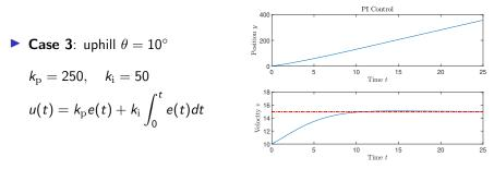
**Disturbance attenuation**: The same PI controller achieves *zero steady-state error*, i.e.,  $e(t) \rightarrow 0$ , despite the presence of an *unknown* disturbance  $\theta$ .
