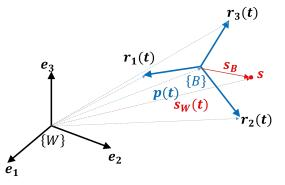
▶ A point **s** on the rigid body has fixed coordinates  $\mathbf{s}_B \in \mathbb{R}^3$  in the body frame  $\{B\}$  but time-varying coordinates  $\mathbf{s}_W(t) \in \mathbb{R}^3$  in the world frame  $\{W\}$
