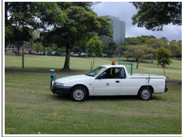
Figure 10: The utility car used for collecting outdoor data is equipped with a SICK laser range and bearing sensor, linear variable differential transformer sensor for the steering and back wheel velocity encoder. This image shows the vehicle in the Victoria Park environment.
