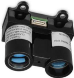
Single-beam Garmin Lidar
