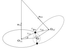
Intersecting circle of spheres with radii z<sub>2</sub> and z<sub>3</sub>: center o<sub>23</sub>, radius r<sub>23</sub>, normal vector n<sub>23</sub> (perpendicular to the circle plane):
