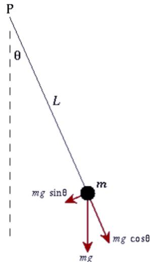
$$\tau = -mgL \sin \theta(t) = mL^2 \ddot{\theta}(t) \quad \Rightarrow \quad \ddot{\theta}(t) = -\frac{g}{L} \sin \theta(t) + \underbrace{w(t)}_{\text{noise} \sim \mathcal{N}(0, q)}$$
