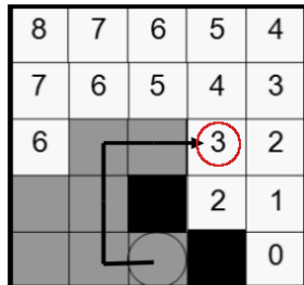
(c) Unexpanded state with smallest f = 5 + 3 = 8
