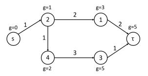
**Path recovery**: once correct g-values are available, the least-cost path  $i_q^*, \ldots, i_1^*$  is a greedy path computed starting from  $i_1^* = \tau$  and backtracking:
