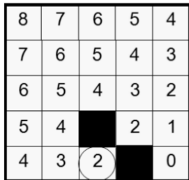
(a) 4-connected grid with Manhattan heuristic
