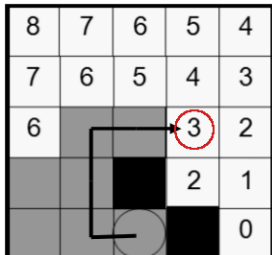
(c) Unexpanded node with smallest f = 5 + 3 value
