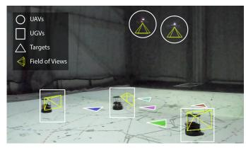
Fig. 1: A real-world dynamic target tracking scenario. Unmanned ground and aerial vehicles (UGVs and UAVs) use onboard cameras to collaboratively estimate the states of moving targets with different colors. The proposed approach is able to coordinate heterogeneous robots with desired trade-off between sensing performance and energy cost, while guaranteeing inter-robot collision avoidance.
