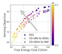
Fig. 7: Trade-off between sensing performance (mutual information (5)) and the true energy expenditure C(S)/m in heterogeneous robot experiments produced by DLS and CD, where it is better to be in the upper left pointed by the gray arrow. Each point is an average obtained over 50 trials for a fixed m, where we set  $m_i = m$  for each robot i to penalize the team energy expenditure per (41).
