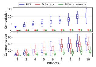
Fig. 5: Computation and communication savings afforded by lazy search (Lazy) and greedy warm start (Warm) for DLS. Computation is measured by total oracle calls divided by the number of trajectories N, where N reaches around 12500 for 10 robots. Communication is measured by the number of proposal exchanges. Combining lazy search and greedy warm start (green) leads to 80–92% computation reduction, and up to 60% communication reduction compared to the naive implementation (blue) on average.
