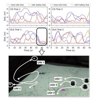
Fig. 16: Collision avoidance constraints are satisfied at all time in all hardware trials, where the inter-UAV and inter-UGV distances never fall below the safety distances (top 4 figures). A particular moment in Trial 1 with DLS is shown at the bottom with robot trajectories overlaid on top, demonstrating safe decentralized navigation.
