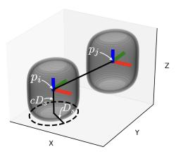
Fig. 3: Illustration of the safe set encoded by the circular superellipsoid barrier function (25) for robots i and j with position  $p_i$  and  $p_j$  respectively. Note that  $D_s$  is the safety radius and  $2cD_s$  is the height of the ellipsoid.
