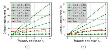
Fig. 5: Collision checking time comparison between our methods and sampling-based (SB) ones with different sampling interval  $\Delta$  for (a) line segments  $\mathbf{p}(t) = \mathbf{p}_0 + \mathbf{v}t$  and (b)  $2^{nd}$ -order polynomial curves  $\mathbf{p}(t) = \mathbf{p}_0 + \mathbf{v}t + \mathbf{a}t^2$  for  $t \in [0, t_f]$  with various values of  $t_f$ .
