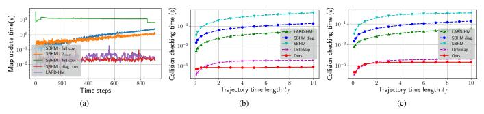
Fig. 7: (a) Map update times and collision checking time comparison for (b) line segments  $\mathbf{p}(t) = \mathbf{p}_0 + \mathbf{v}t$  and (c) second-order polynomial curves  $\mathbf{p}(t) = \mathbf{p}_0 + \mathbf{v}t + \mathbf{a}t^2$  for  $t \in [0, t_f]$  with various values of  $t_f$ . Our proposed collision checking described in Sec. VI is used with our SBKM map while sampling-based collision checking with sampling resolution  $\Delta = 0.005$  is used with the other maps.
