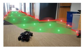
Fig. 1: A ground robot in an unknown environment relying on lidar scan data (red) for online occupancy mapping and collisionfree trajectory planning. Our mapping algorithm learns a sparse set of occupied and free relevance vectors (light red and green dots, respectively) that represents the environment based on the lidar scans.
