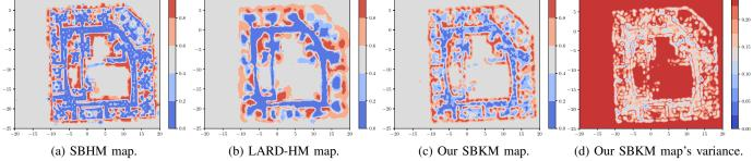
Fig. 6: Comparison among our sparse Bayesian kernel-based map (SBKM), Localized Automatic Relevance Determination Hilbert Map (LARD-HM) [36] with 7280 clusters, and Sequential Bayesian Hilbert Map (SBHM) [35] with  $\eta = 1$ ,  $\Gamma = \sqrt{6.71}I$  built online using lidar scans from the Intel Research Lab dataset [63].
