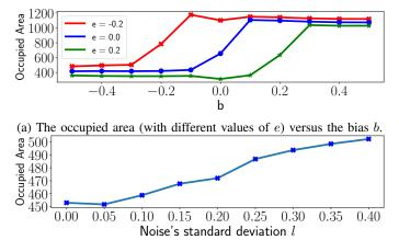
(b) The occupied area (with b = -0.01, e = 0.0) versus the noise's standard deviation.
