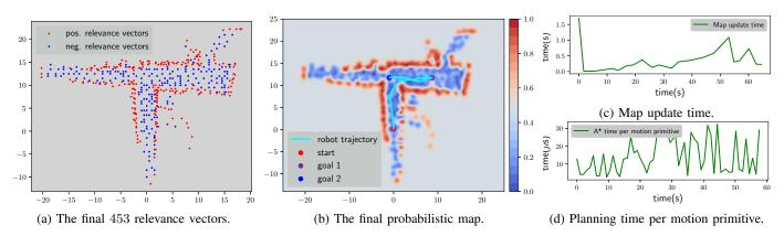
Fig. 9: Real experiment with an autonomous Racecar robot navigating in an unknown hallway environment: (a) The final 453 relevance vectors; (b) The final probabilistic map; (c) Map update time; (d) Planning time per motion primitive. Please refer to our website https://thaipduong.github.io/sbkm for the experiment video.
