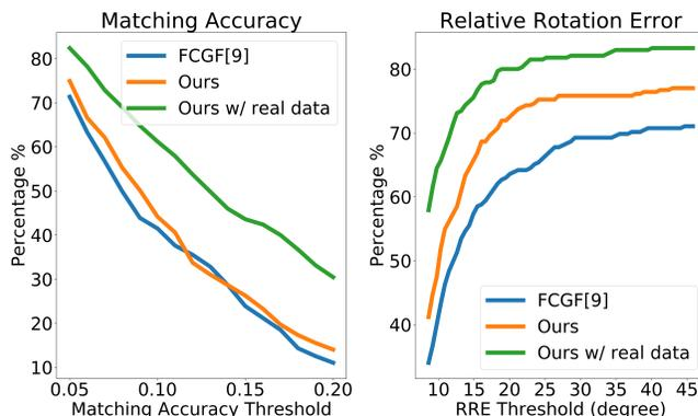
Fig. 7: Results on ScanNet real-world data. Left: matching accuracy. Right: relative rotation error. FCGF [5] is the baseline model w/o cross-instance matching. Our w/ real data is the model trained with real-world point clouds.
