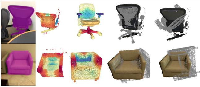
Fig. 9: Failure cases on RGB-D point cloud registration. Column 1: RGB images and object segmentation masks in purple. Column 2 & 3: color-coded point cloud features of the observed objects and the CAD models. Column 4 & 5: Different alignment results after running RANSAC, with the CAD models painted in grey.
