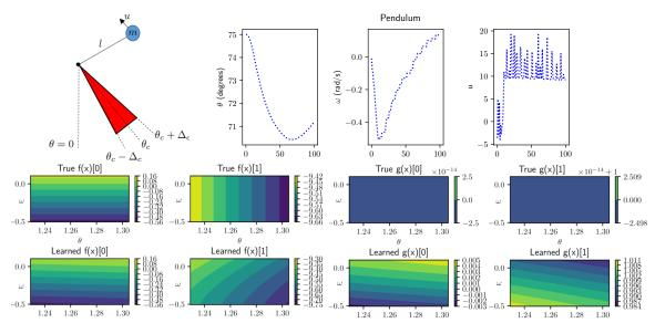
Figure 1: **Top left**: Pendulum simulation (left) with an unsafe (red) region. **Top right**: The pendulum trajectory (middle) resulting from the application of safe control inputs (right) is shown. **Bottom row**: Learned vs true pendulum dynamics using matrix variate Gaussian Process regression
