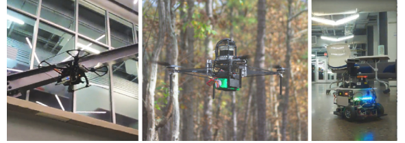
Figure 1: Robot platforms used in our experiments. We utilize three types of robots for our experiments: two aerial platforms, the Falcon 250 UAV (left) and the Falcon 4 UAV (middle), and one ground platform, the Scarab UGV (right). The Light Detection and Ranging (LiDAR)-equipped robot (Falcon 4) is primarily used for outdoor operations due to its size and superior sensing capabilities. The RGB and Depth (RGBD) camera-based robots (Falcon 250 and Scarab) are more suitable for cluttered indoor environments due to their smaller footprints. All three platforms have GPS-denied autonomous navigation capabilities, enabling them to safely explore cluttered environments using only onboard computation and sensing.
